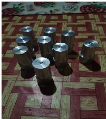
Fig. 10 Aluminum 6061 specimens after turning.
