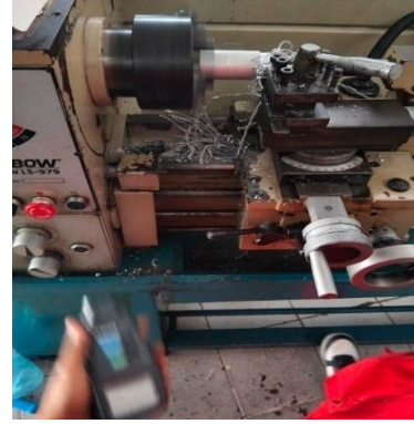
Fig. 9 Turning operation on the conventional lathe.
