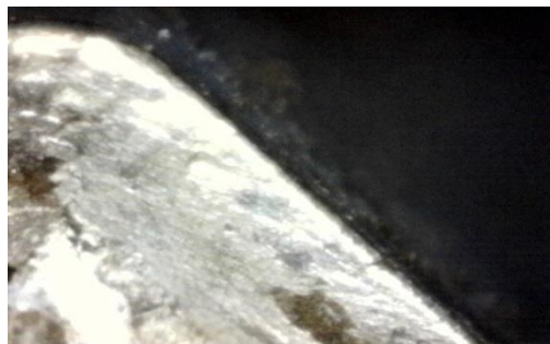
Fig. 12 Carbide flank face observed using a digital microscope.
