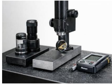
Fig. 6 Optical microscope and digital measuring equipment used for flank-wear observation.
