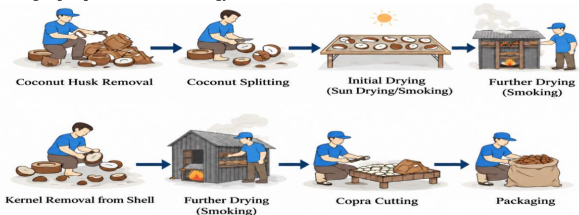
Fig. 1. Observed household-scale copra processing sequence in Buton Regency.
