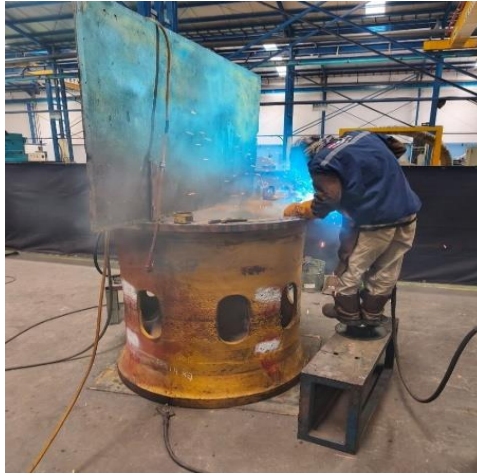
Fig. 1. Condition of plug welding activity on the Rear Wheel Hub component
